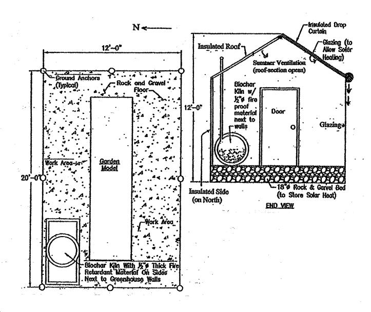
This kiln is designed to produce biochar while also accomplishing cooking of foods and generation of electricity by thermoelectric means. Steel used for drums must not be galvanized. The concept assumes villagers will share biochar making & cooking tasks, while also sharing electricity produced.
